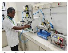
Specifications: Make : VB Ceramic consultants Shell design: Suitable for vacuum and pressure (1mbar) Maximum temperature:  $600^{\circ}C$  (accuracy  $\pm 1^{\circ}C$ ) Rotary vacuum pump (10<sup>-1</sup> mbar) Mass flow controller
