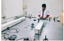
Specifications: Brand : Litron Lasers Laser medium : Nd-YAG Laser Energy - 400 mJ Laser Wavelength - 1064nm Pulsed duration - 6ns
