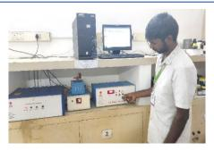
Specifications: Brand: Marine India Maximum Field: +5KV/(50KV/cm) Frequency Range: 20Hz – 1 KHz Cryogenic Temperature Stage: 100RT (96K – 273K) Sample Dimension: 2 - 10 mm diameter
