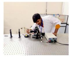
Specifications: Make : THOR Labs Laser-Nd-YAG Laser (1064 nm)
