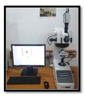
It will be operated by putting a controlled force on the surface of the material over a period of time. After a particular indenter is pressed into the surface under testing, the indentation resulting from it is measured and the software is also used to analyze and generate precise results.
