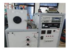
Specifications: Brand : VacuTech Systems Two sputtering guns (DC and RF) Maximum power 300 W Temperature: 500°C Base pressure: 1 × 10<sup>-6</sup> mTorr
