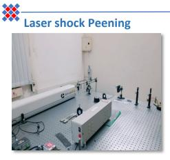
**Specifications:** Litron Lasers Medium :(Nd-YAG Laser, 400 mJ) Wavelength: 1064nm Pulse Width : 6nsec
