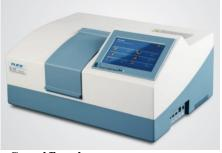
Specifications : Brand : ELICO Model : SL218 Deuterium Lamp (D<sub>2</sub>) Tungsten (W) Halogen Lamp
