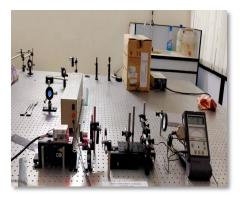
Z-scan technique is used to measure the nonlinear optical properties of materials. The Z-Scan helps to determine intrinsic photo-physical properties of materials by focusing a single laser beams onto the surface of the materials sample. Usually, measurements need to be taken at different laser pulse energies or different laser pulse lifetimes in order to determine what nonlinear processes are present.
