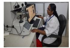
Specifications: Make and Model: Mitutuoyo-HB210 Indent: Diamond Indenter Magnification: 10x and 50x Vicker's hardness and Knoop Hardness, Load: 10 to 1000 kgf (load applied for 10 to 15 seconds)
